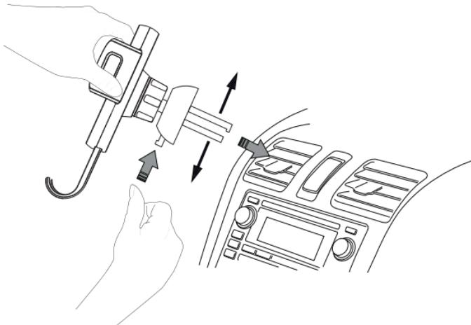
**3****Installation of the smartphone into the holder**
