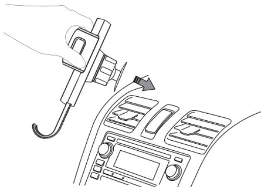
**2****Installation of the holder on the air vent grille**
