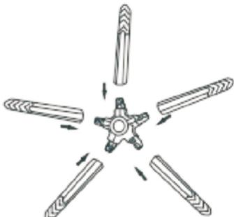
**2. Push and twist the casters into the star base. Place the gas lift into the star base. Place the gas lift cover over the gas lift.**
