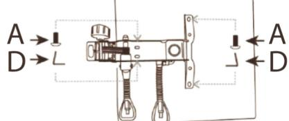
**4. Secure the footrest 11 with the screws B on the footrest support on the bottom of the seat 2.**
