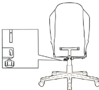
**8. Fasten the armrests with screws C. Close the screw holes with caps E.**
