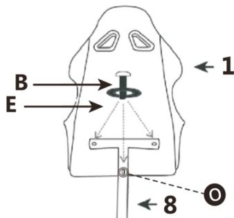
**6. Insert the backrest mount into the hole in the butterfly mechanism and secure it by turning the handle.**
