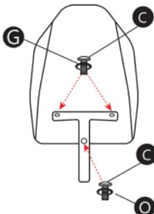
**7. Insert the backrest mount into the hole in the butterfly mechanism and secure it by turning the handle.**
